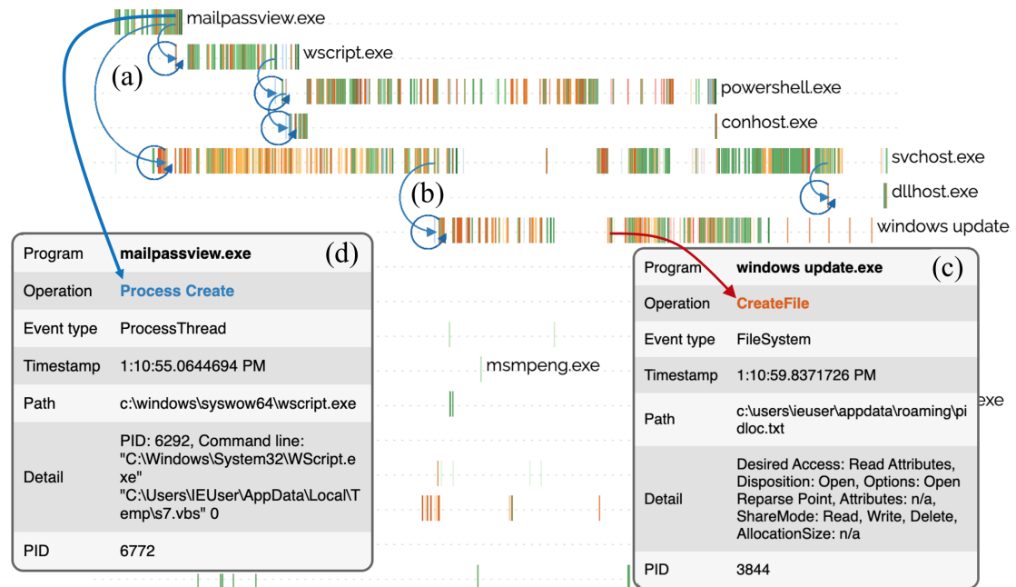
Figure 5.10: MalView view on a Hacktool malware type called Mailpassview . It first creates process svchost.exe (a), then svchost.exe starts windows update.exe (b), and then windows update.exe creates pidloc.txt (c)
